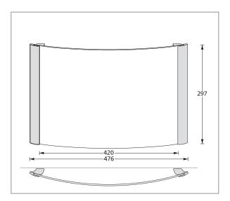
The size of the wall-mounted signposts 3042 correspond to the size DIN A3 landscape. The axis dimension is important for mounting the profiles on the wall, it indicates the distance between the wall holes. The axis dimension for signposts in the 540 module grid is 522 mm. Article number with painted profiles: SWO 3042 L
